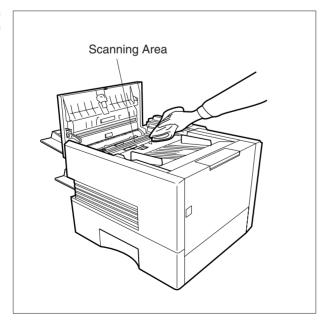
Wipe the Scanning Area gently with a soft cloth gauze wet with ethyl alcohol. Be sure to use a clean cloth, the scanning area can be easily scratched.
